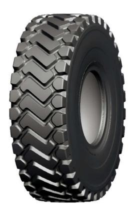
Standard L3 rock lug pattern combines excellent traction and high resistance to wear and cutting.
